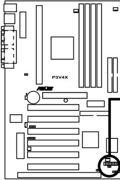
**TIP:** If the case-mounted LED does not light, try reversing the 2-pin plug.
