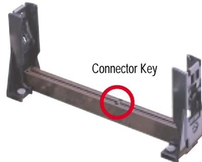
2. Push down firmly but gently the SECC2/SECC/SEPP into the URM until it snaps into place.
