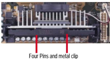
**NOTE:** The SEPP heatsink and fan (for Intel Celeron processors) is similar to the SECC2 heatsink and fan except that the clamping design is different.
