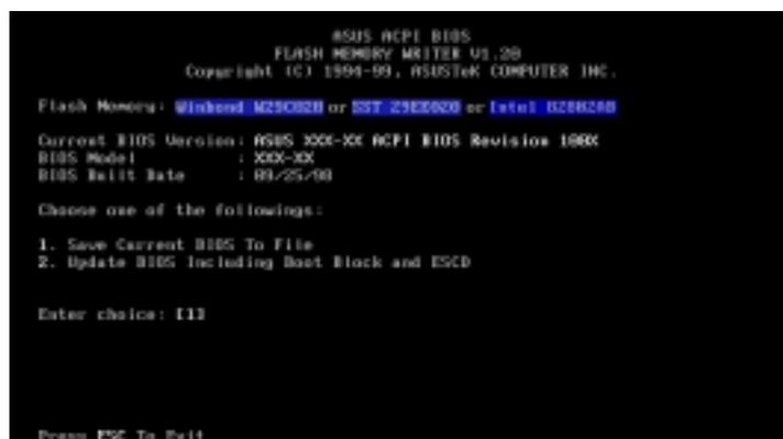
**IMPORTANT!** If “unknown” is displayed after **Flash Memory:**, the memory chip is either not programmable or is not supported by the ACPI BIOS and therefore, cannot be programmed by the Flash Memory Writer utility.
