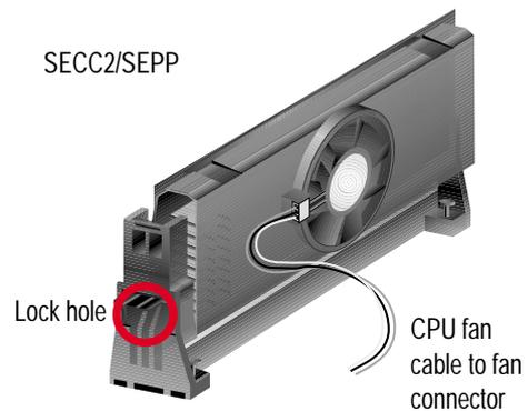
3. If your URM is of type A, make sure the locks are in the locked position as shown.
